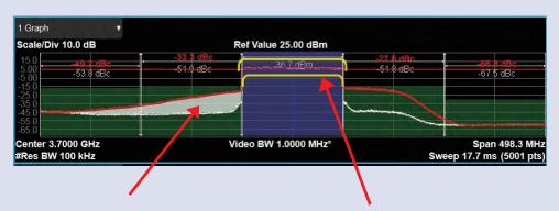
Crest Factor Reduction (CFR) reduces over-the-air distortion of PA
